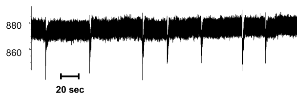
Figure 12. Current-time transient for a PEG-functionalized conical nanotube sensor with a solution 100 nM in BSA and 270 nM in anti-BSA-Fab on the tip side of the membrane. Tip diameter = 17 nm. Transmembrane potential = 1000 mV.
